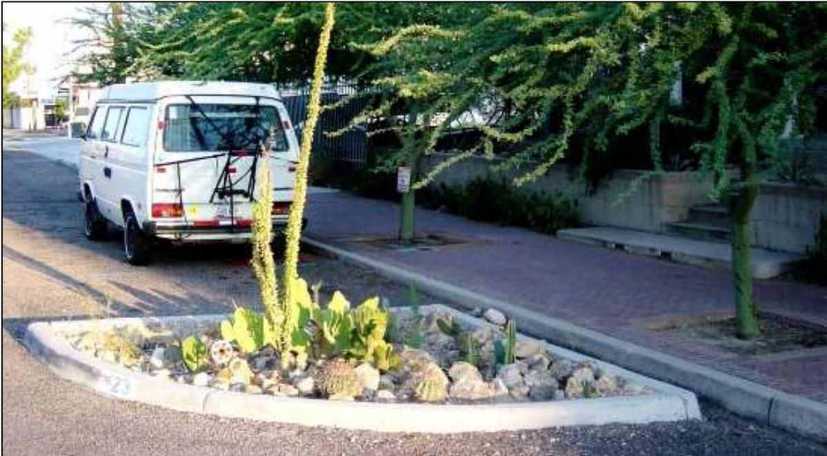
Old style curb extension built by the City as part of the Stone Avenue improvements does not have curb openings to allow water to flow into the landscaped basin. Avenue.
